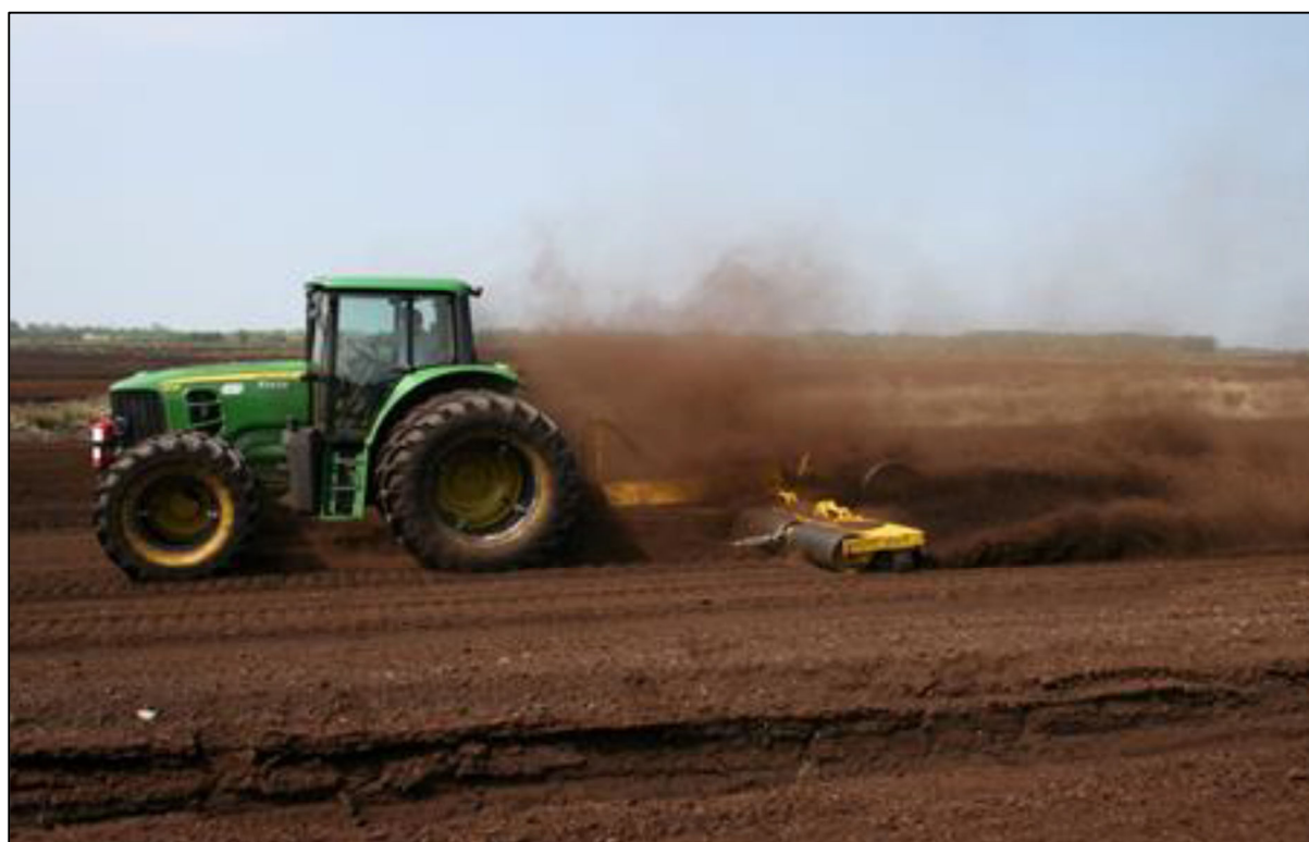
Plate 4-8: Milling process (source: Bord na Móna)
