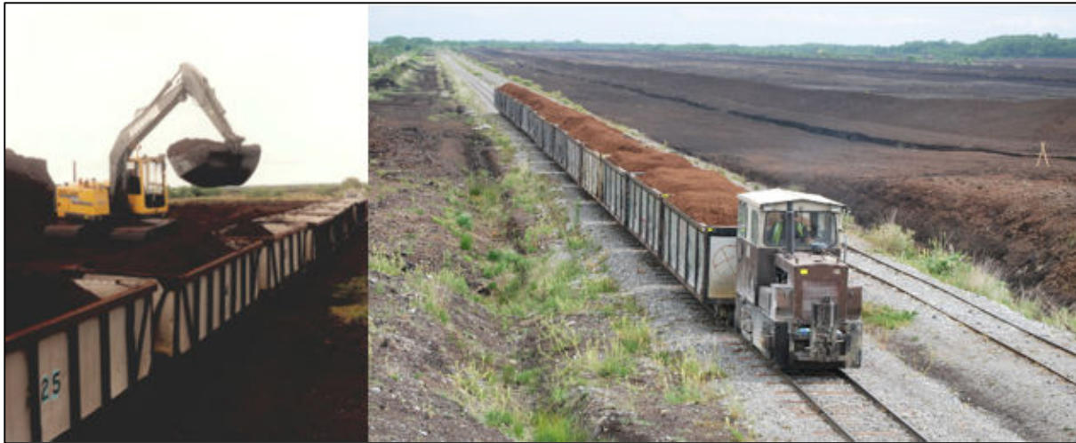
Plate 4-38: Example of railway locomotive and wagons hauling milled peat to the power plant (source: Bord na Móna)
