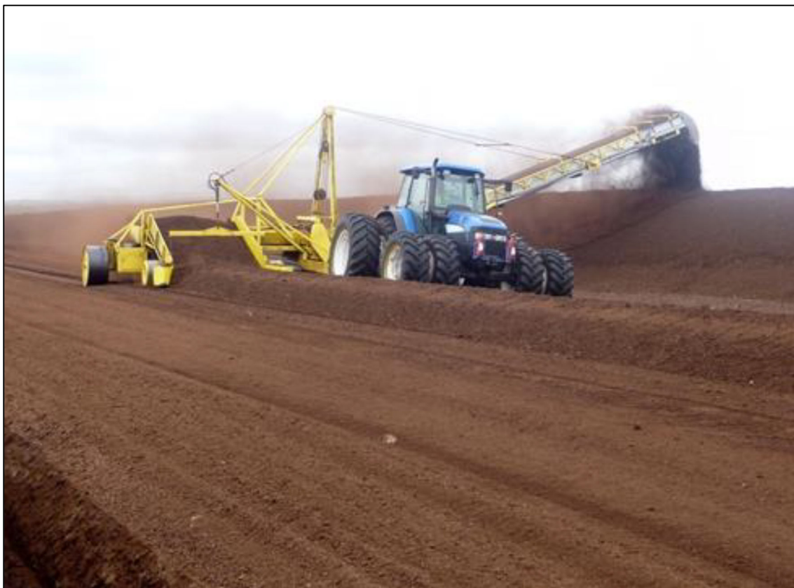
Plate 4-12: Harvesting - Peco Method (source: Bord na Móna)
