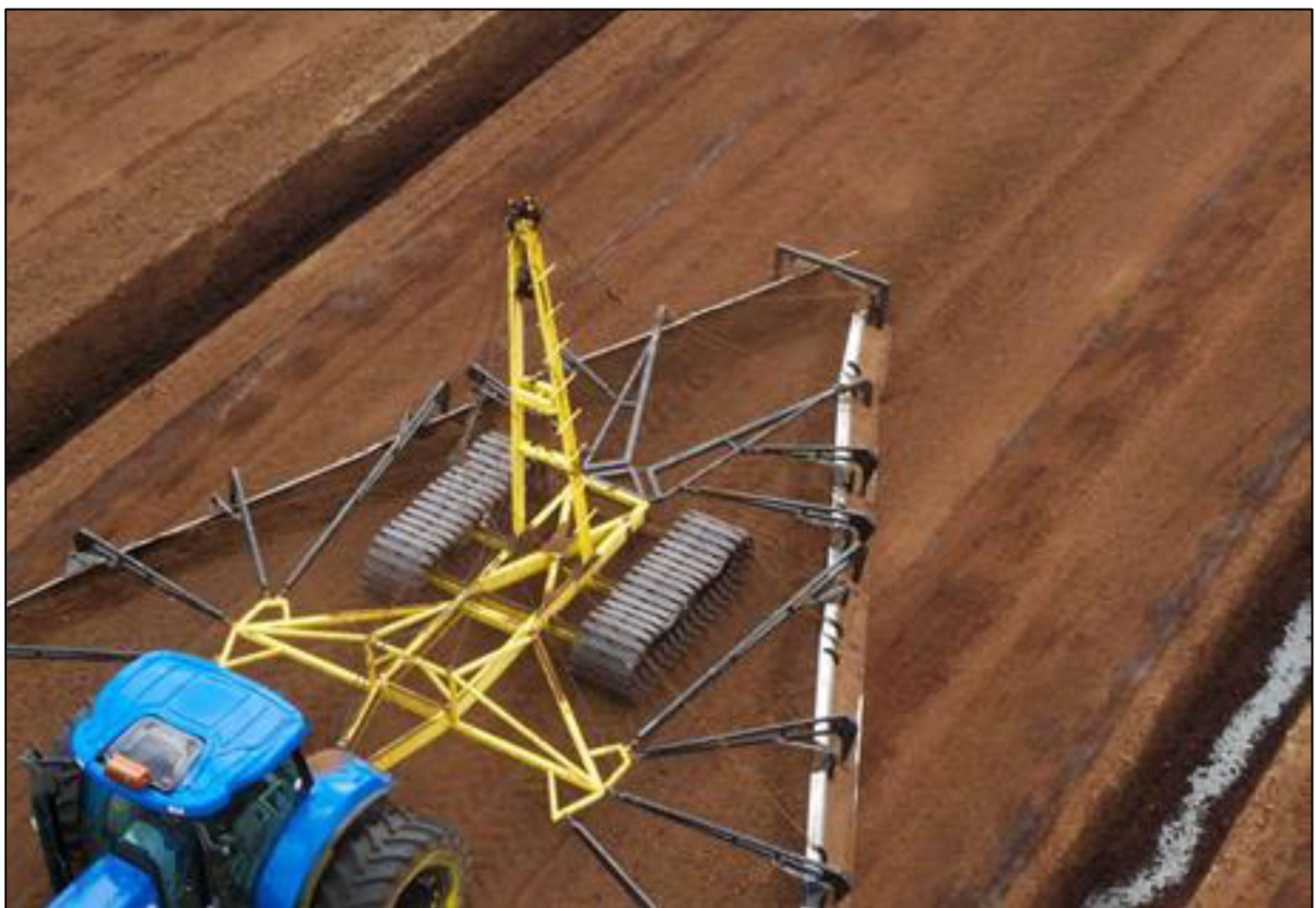
Plate 4-10: Ridging process (source: Bord na Móna)
