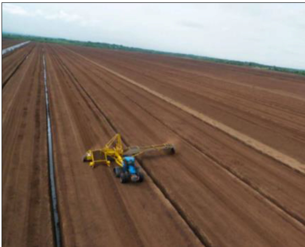
Plate 4-13: Harvesting – Peco method (source: Bord na Móna)
